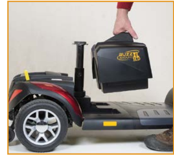
Step 2: Pull out the battery pack!
