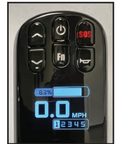
Controller is pre-wired allowing right or left side placement
